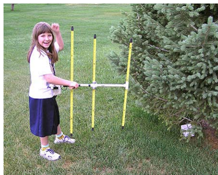
KE7DRD finds her first hidden transmitter with a homebrew RDF device.
